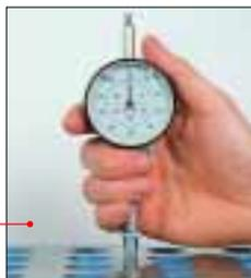
The required tolerance range is set on the dial in the normal way. In our example:  $\pm 10$ .
