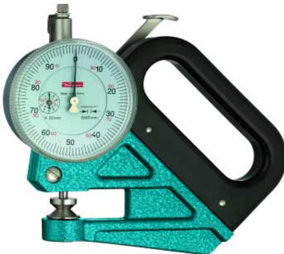
The predecessor model F 1000/30 of the new Foil Dial Thickness Gauge F 1101/30 is still available. One revolution of the pointer equals 0,2 mm corresponding to 200 graduations. Its measuring pressure is approximately 2 N. If required it can be supplied with a higher measuring force of 4,5 N or with a lower measuring force of 1,2 N.
