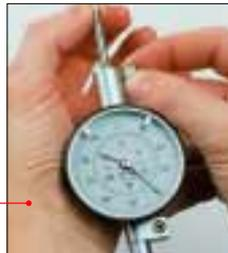
Move the measuring stop over the tool loosely secured in the clamping unit and push it inwards until it has engaged properly. The tool will be positioned with the required projection.
