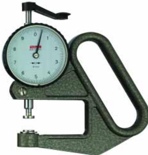
Model K 50 with lifting device has the same technical specification as model K 50 with pressure lever. At rest the feelers are closed. This style has the advantage that the contact pressure of 0,5 N is applied independently of the user. The Spare Dial Gauge for K 50 with lifting device will be supplied without lifting device unless requested on the order.
