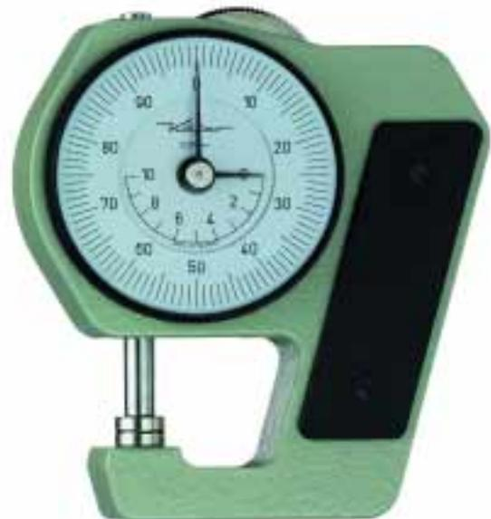
The feelers are in contact when the Pocket Dial Thickness Gauges J 12 and J 15 are not in use. The serrated lifting wheel opens them for the insertion of the component. The size can be easily read off the scale. The instruments can be zeroed by using the knurled adjusting bezel.
