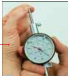
Clamp the measuring pin with the help of the pre-setting screw.
